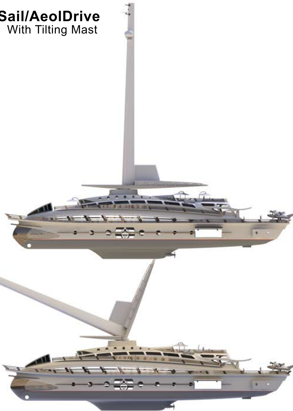
Air-draft reduced from 237' to 134' for bridge clearance
